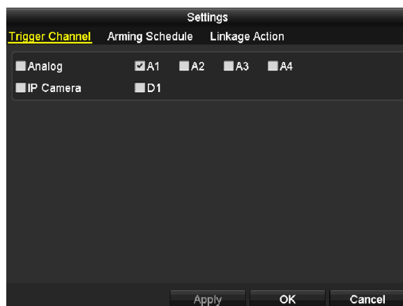
Figure 8.15 Set Triggering Channel of VCA Alarm
